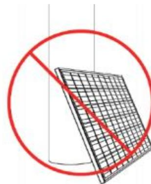
4.2.9 If all the modules are NOT removed after unpacking and some of them are left in the package, the remaining modules shall be laid flat and repackaged to prevent from falling down. Must be placed by horizontal. The stacked number of modules: Stacked NO MORE than 16 pieces.
