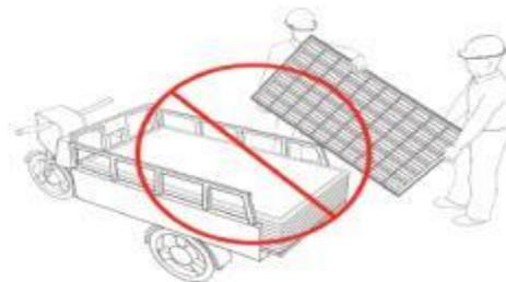
3.3.7 Do Not transport the modules with rope as shown below:
