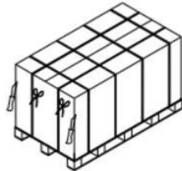
4.2.5 Cut the tape at shorter edge and hold it up by 90° from the bottom; and pull out the cardboard to expose the modules.
