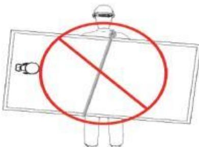
3.3.8 Do Not carry the modules on the back of one person as shown below:
