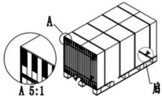
4.2.7 When unpacking on a level surface, take out the module from one side of package to the other, and then carry it with two persons (Please refer to 3.1.8) When unpacking on a sloping surface, please protect the modules from tipping over or sliding. As shown below.
