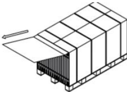
4.2.6 Cut the two horizontal packing belts in the carton and cut the two packing belts near the bottom of the tray, and remove the packing belts
