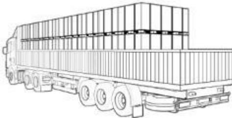
3.3.4 Only one layer stacking is only allowed for small truck. Make sure that the package is fixed with packing straps securely to the shipping platform without movement.
