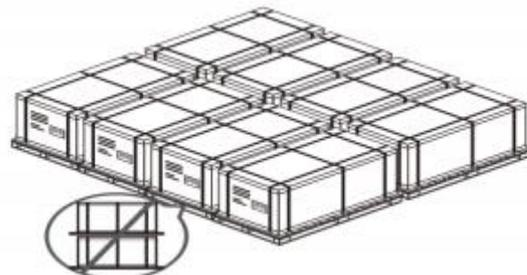
3.2.5 Cover all of parts of the package with waterproof material to prevent the panel package and plate from moisture.
