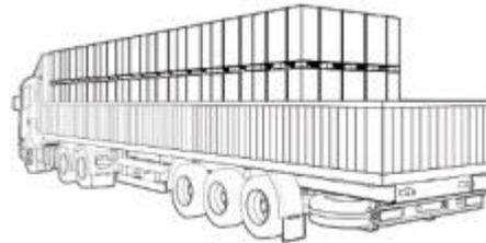
3.3.3 Transport: Do Not Stack more than two layers on truck.
