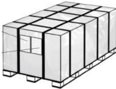
4.2.4 Cut the two packing belts at shorter sides of the tray with blade or scissors, and unpack the side surface of the carton along the vertical direction.
