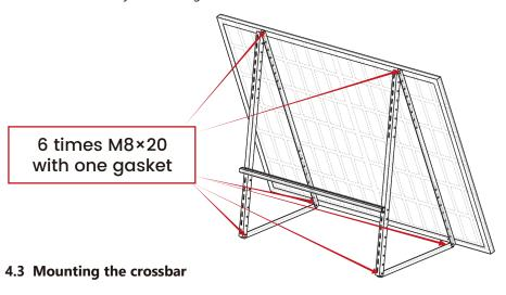
The crossbar gives the additional stability of the substructure and is usually used to mount the micro-inverter directly. When doing so, observe the required cable lengths.
