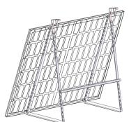
Scheme of hook fastening on the balcony with adjustable angle from 27 ° to 41 °.
